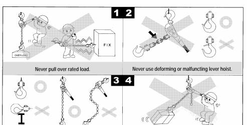
Never use the load chain to wrap the pulling object and never use when top hook and lower hook do not in line.
