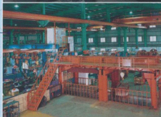
• Wire Rope Hoist Load Test Platform • All Hoist Must Pass 125% Load Test Prior To Shipment
